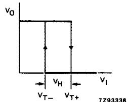
Fig.6 Transfer characteristic.
