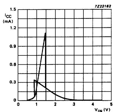
Fig.11 Typical HCT transfer characteristics;  $V_{CC} = 4.5$  V.
