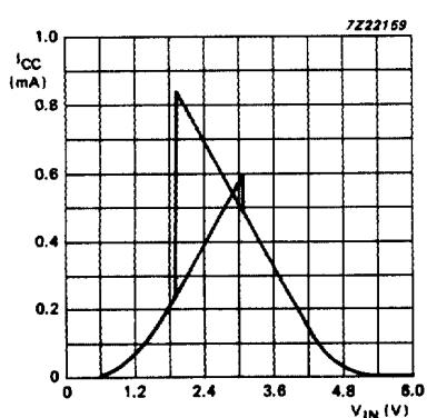
Fig.10 Typical HC transfer characteristics;  $V_{CC} = 6$  V.
