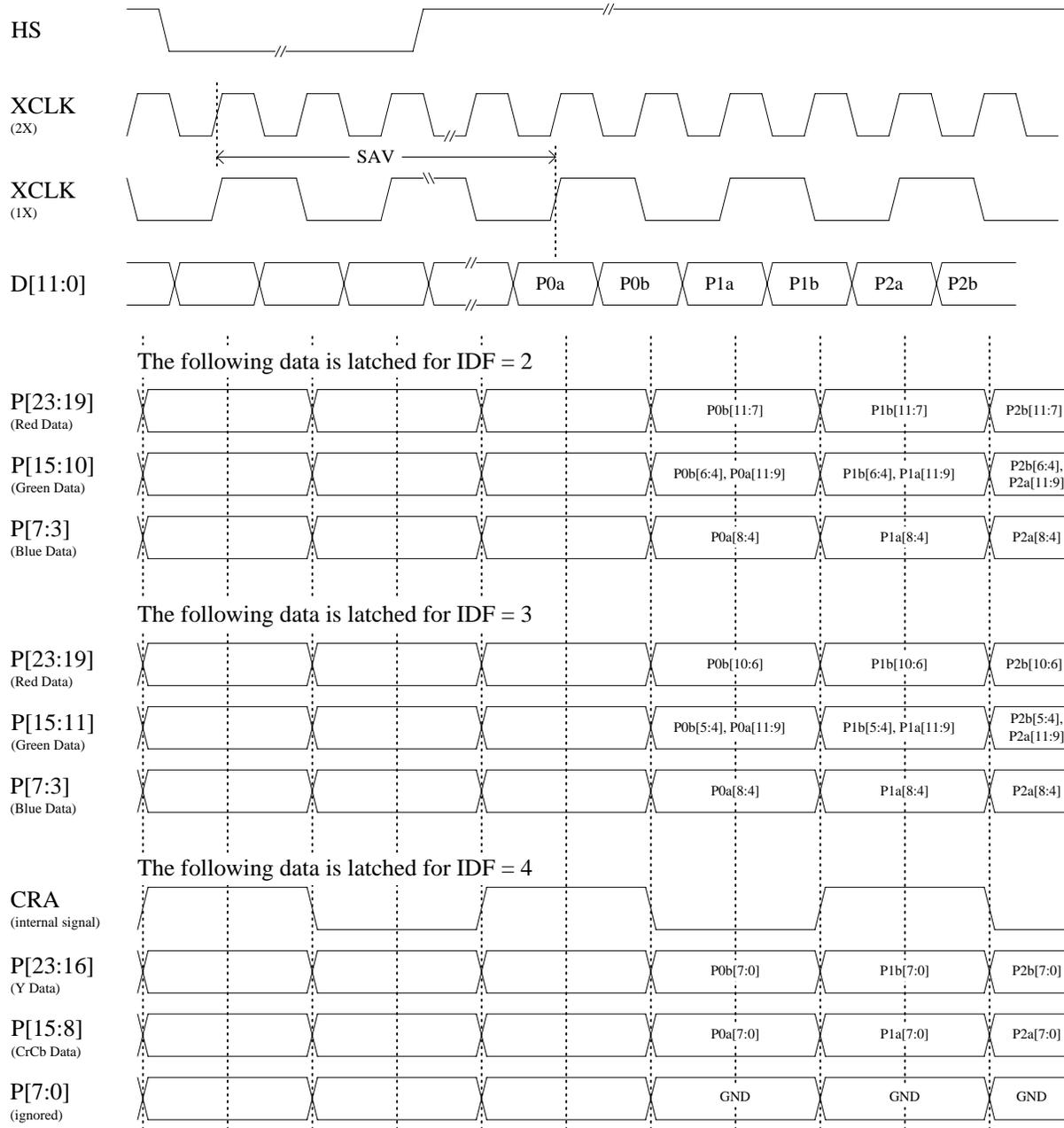
Figure 5. Multiplexed Input Data Formats (IDF = 2, 3, 4)
