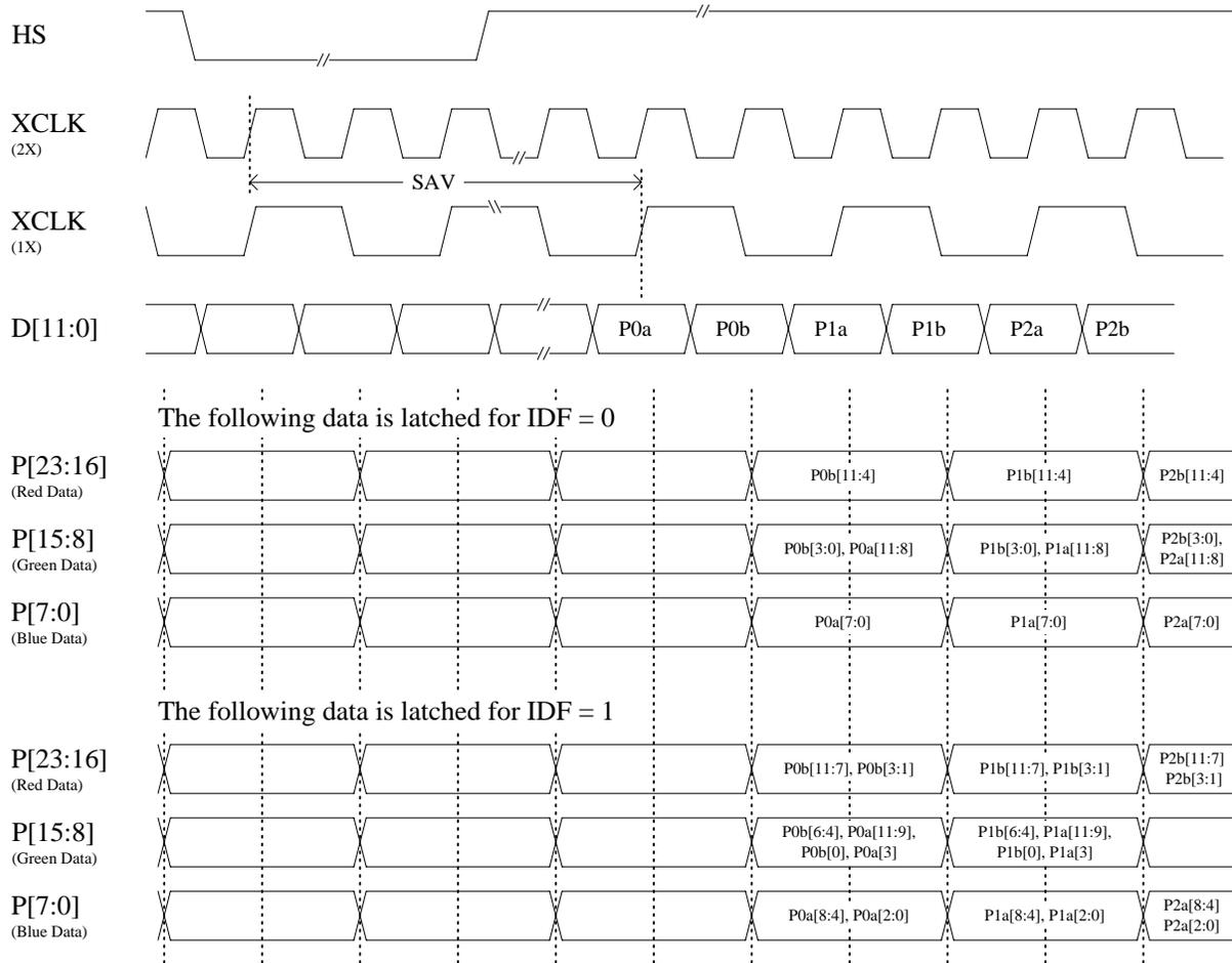
Figure 4. Multiplexed Input Data Formats (IDF = 0, 1)
