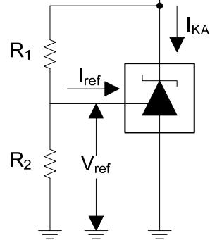
Test Circuit for  $V_{KA} = V_{ref}(1+R_1/R_2)+R_1 \cdot I_{ref}$
