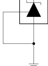
Test Circuit for  $I_{off}$
