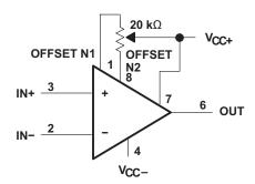
Figure 1. Input Offset-Voltage Null Circuit
