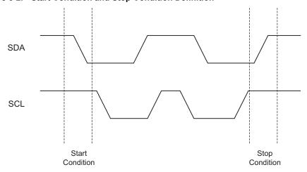
**Stop Condition:** A low-to-high transition of SDA with SCL high is a Stop condition. After a Read sequence, the Stop condition will place the EEPROM in a standby power mode (See Figure 6-2).
