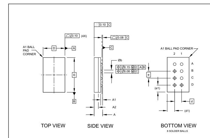
COMMON DIMENSIONS (Unit of Measure = mm)
