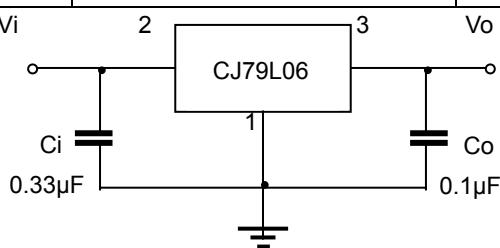
Note: Bypass capacitors are recommended for optimum stability and transient response and should be located as close possible to the regulators.
