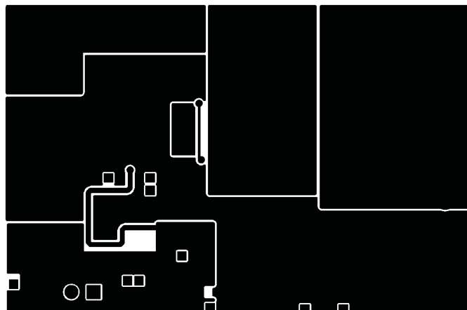
Figure 43. TPS40200EVM-001 Bottom Copper (X-Ray View from Top)
