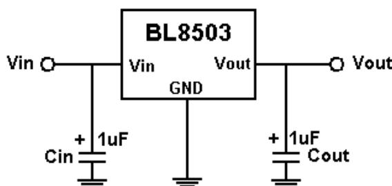
NOTE1 : Input capacitor ( $C_{in}=1\mu F$ ) is recommended in all application circuit. Tantalum capacitor is recommended.
