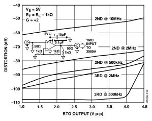
Figure 19. Harmonic Distortion vs. Output Signal Amplitude
