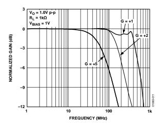
Figure 11. Large Signal Frequency Response
