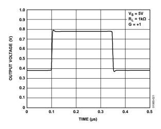
Figure 21. 400 mV Pulse Response
