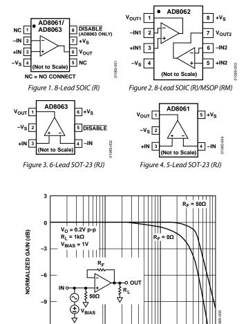
Figure 5. Small Signal Response,  $R_F = 0 \Omega$ , 50  $\Omega$
