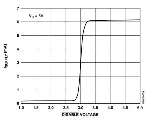
Figure 34. AD8063 DISABLE Voltage vs. Supply Current
