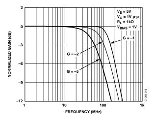
Figure 13. Large Signal Frequency Response
