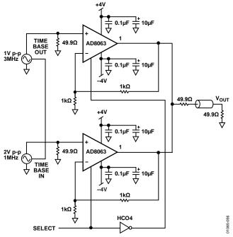
Figure 56. Two-to-One Multiplexer Using Two AD8063s
