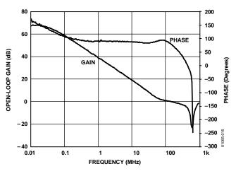
Figure 15. AD8062 Open-Loop Gain and Phase vs. Frequency,  $V_{\rm S}$  = 5 V,  $R_{\rm L}$  = 1 k $\Omega$
