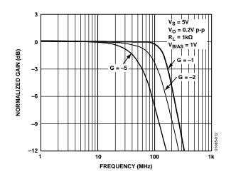
Figure 12. Small Signal Frequency Response
