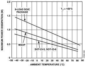
Figure 6. Maximum Power Dissipation vs. Temperature for AD8061/AD8062/AD8063
