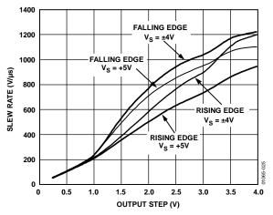
Figure 25. Slew Rate vs. Output Step Amplitude, G = 2,  $R_L = 1$  k $\Omega$ ,  $V_S = 5$  V
