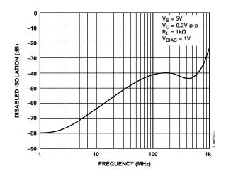
Figure 33. AD8063 Disabled Output Isolation Frequency Response
