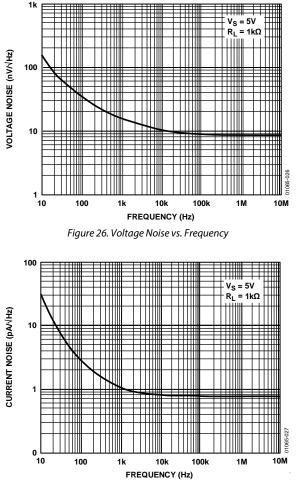
Figure 27. Current Noise vs. Frequency
