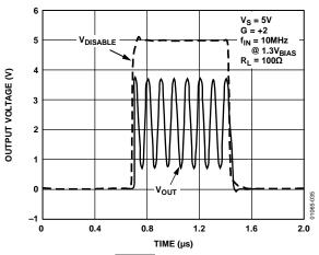
Figure 35. AD8063  $\overline{\text{DISABLE}}$  Function, Voltage = 0 V to 5 V
