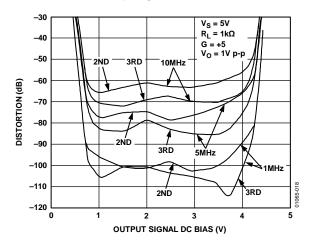
Figure 18. Harmonic Distortion vs. Output Signal DC Bias
