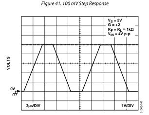
Figure 42. Output Rail-to-Rail Swing
