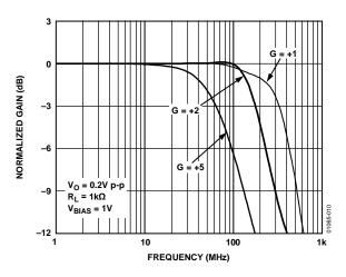
Figure 10. Small Signal Frequency Response
