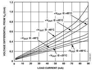
Figure 7. Output Saturation Voltage vs. Load Current
