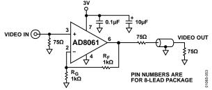
Figure 53. Single 3 V Sync Stripper Using AD8061
