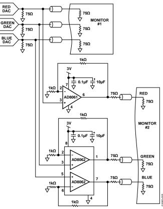
Figure 55. RGB Cable Driver Using AD8061 and AD8062
