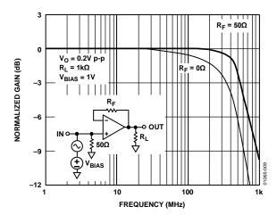
Figure 9. Small Signal Response,  $R_F = 0 \Omega$ , 50  $\Omega$
