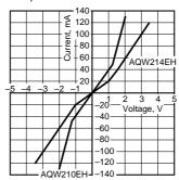
9. Off state leakage current
