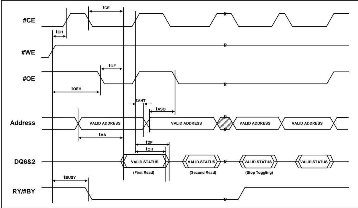
Figure 8-22 Toggling Bit Timing Waveform (During Automatic Algorithms)
