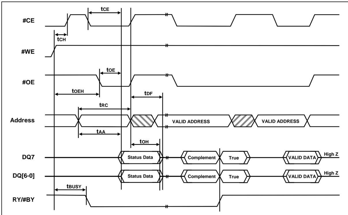
Figure 8-19 Data# Polling Timing Waveform (During Automatic Algorithms)
