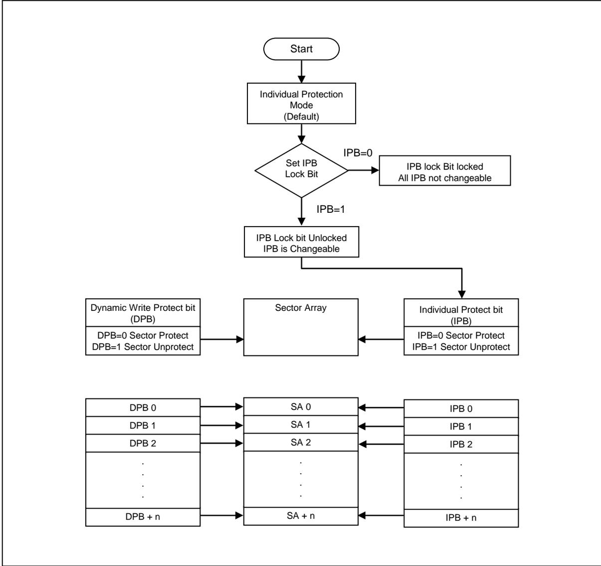
Figure 7-1 Enhanced Sector Protect/Un-protect IPB Program Algorithm
