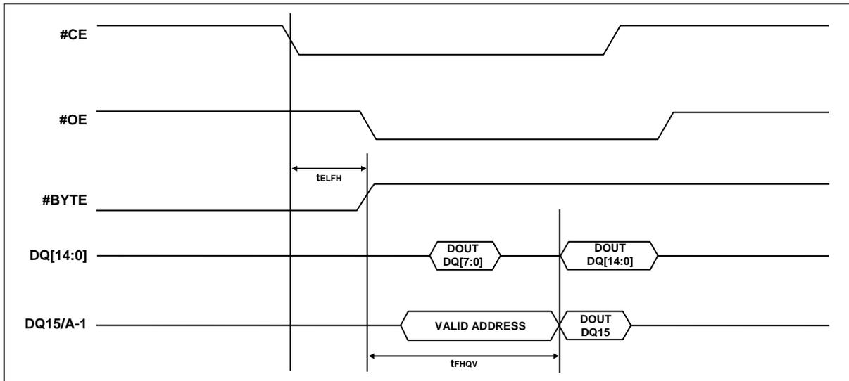
Figure 8-24 #BYTE Timing Waveform For Read operations
