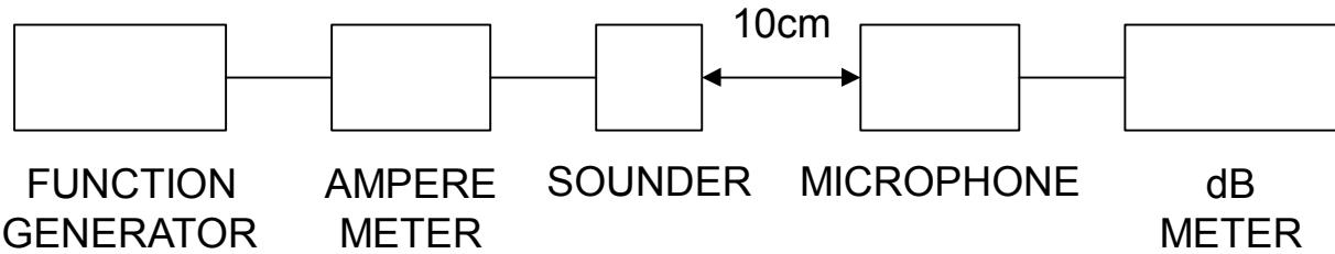
In the measuring test, buzzers is placed as follows:
