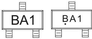
Solid dot = Green molding compound device, if none, the normal device.
