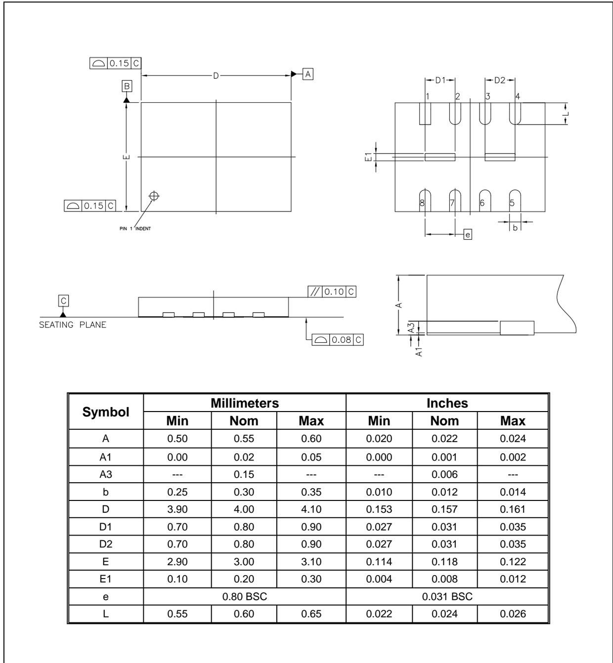
Note: The metal pad area on the bottom center of the package is not connected to any internal electrical signals. It can be left floating or connected to the device ground (GND pin). Avoid placement of exposed PCB vias under the pad.
