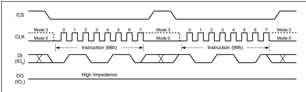
Figure 38. Enable Reset and Reset Instruction Sequence
