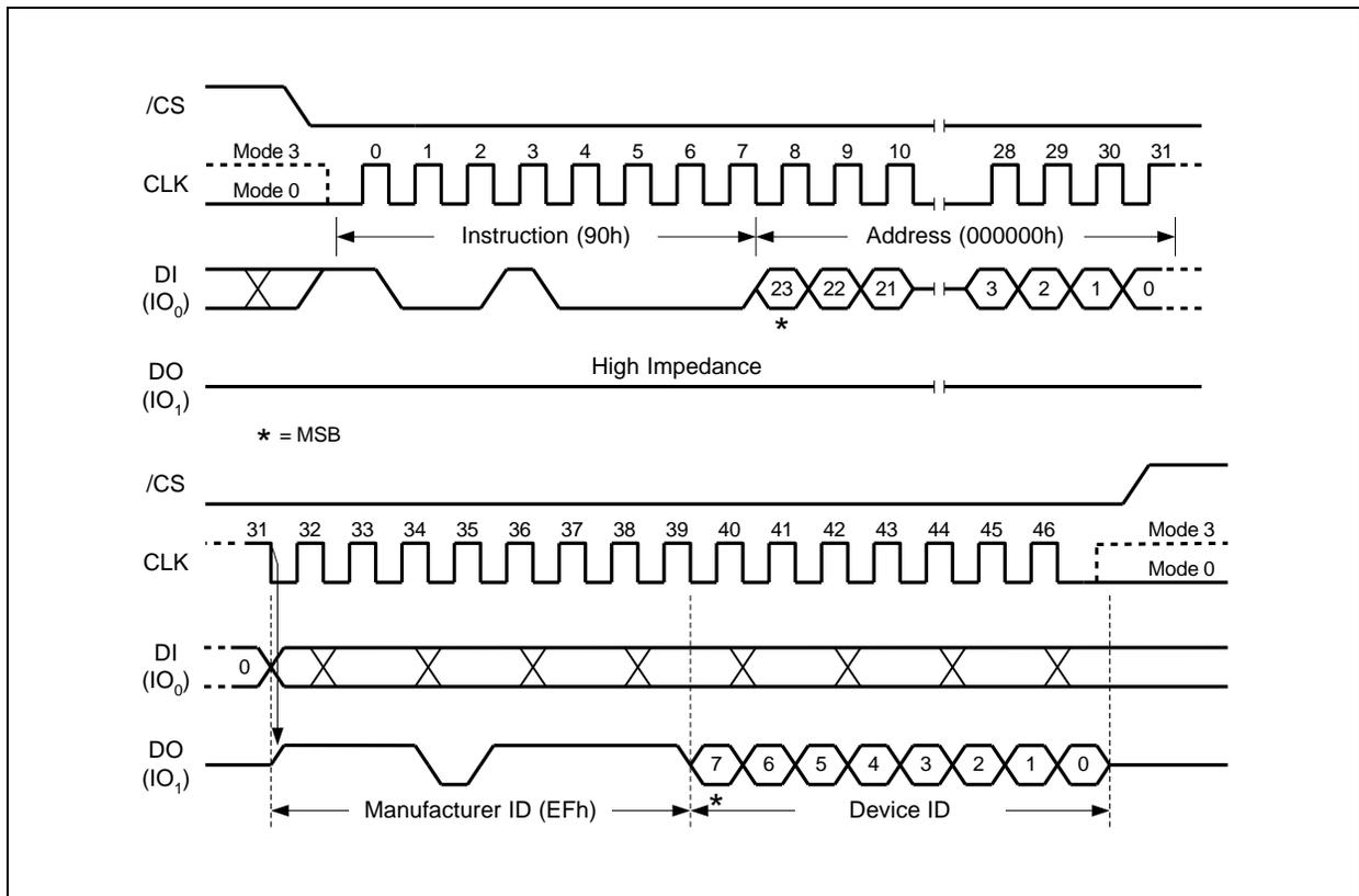
Figure 29. Read Manufacturer / Device ID Diagram
