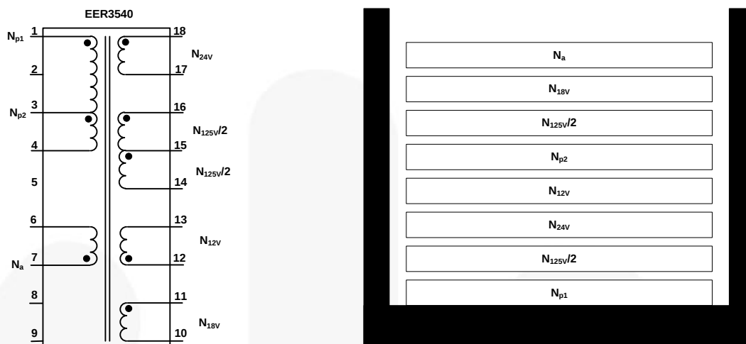
Figure 44. Transformer Schematic Diagram
