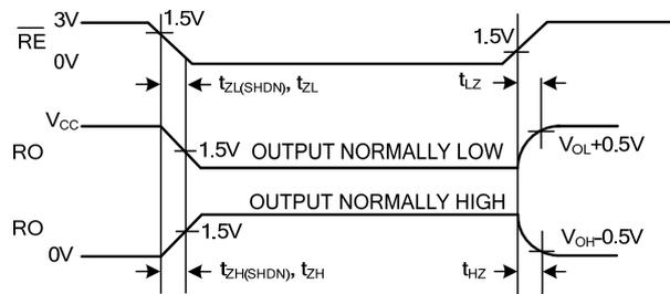
Fig. 8 Receiver Enable and Disable Times
