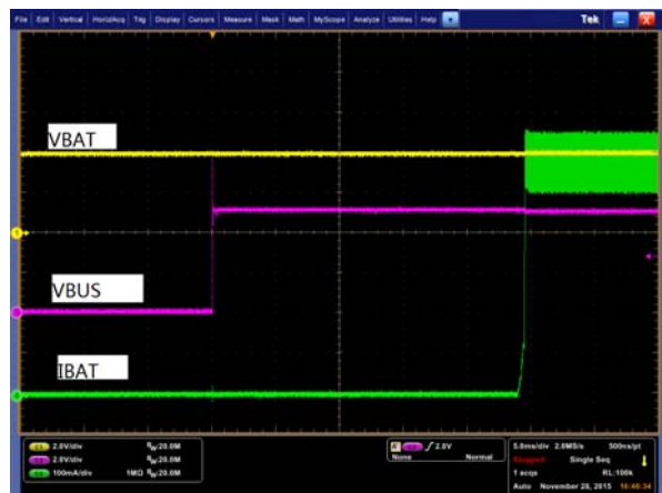
Figure 12. Auto-Charge Startup at V_{BUS} Plug-in, I_{INLIM}=500mA , V_{BAT}=3.9V
