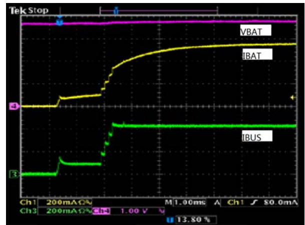
Figure 14. Charger Startup with HZ_MODE Bit Reset, I_{INLIM}=500mA , I_{OCHARGE}=956mA , O_{REG}=4.2V , V_{BAT}=3.6V
