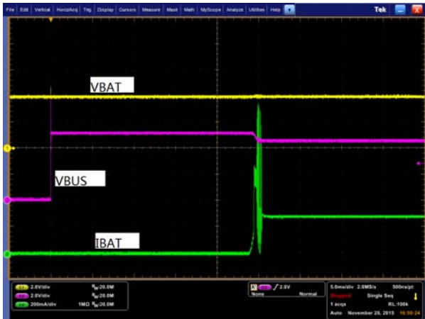
Figure 13. Auto-Charge Startup with 300mA Limited Charger/Adaptor, I_{INLIM}=500mA , V_{BAT}=3.9V
