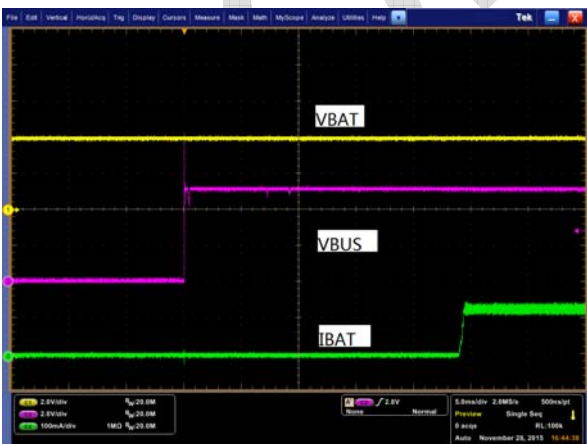
Figure 11. Auto-Charge Startup at V_{BUS} Plug-in, I_{INLIM}=100mA , V_{BAT}=3.9V
