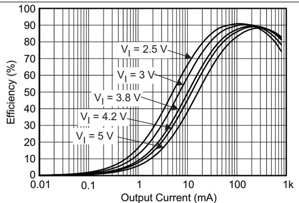
Figure 6. DCDC3: Efficiency vs Output Current
