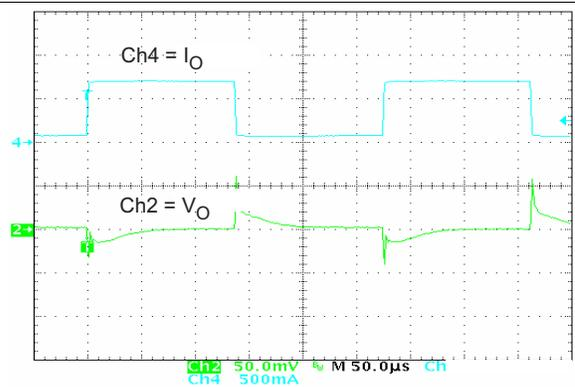
Figure 14. VDCDC3 Load Transient Response
