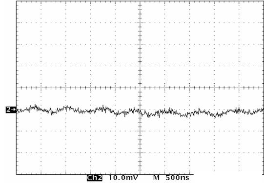
Figure 16. VDCDC2 Output Voltage Ripple
