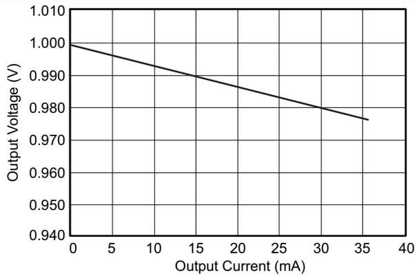
Figure 17. VDD\_ALIVE Output Voltage vs Output Current
