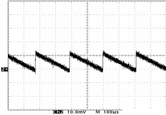
Figure 15. VDCDC2 Output Voltage Ripple
