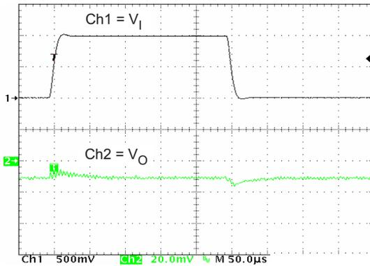
Figure 11. VDCDC3 Line Transient Response
