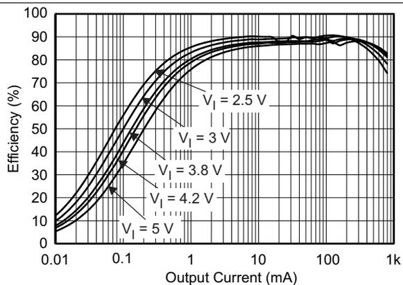
Figure 5. DCDC3: Efficiency vs Output Current
