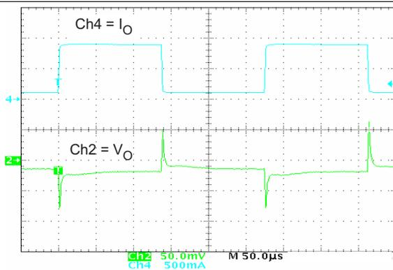
Figure 13. VDCDC2 Load Transient Response
