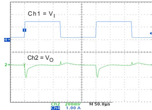
Figure 12. VDCDC1 Load Transient Response
