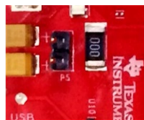
Figure 14. Current Measurement Point
