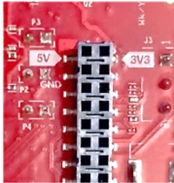
**Figure 8. 3V3 and 5V Marking on BoosterPack**
