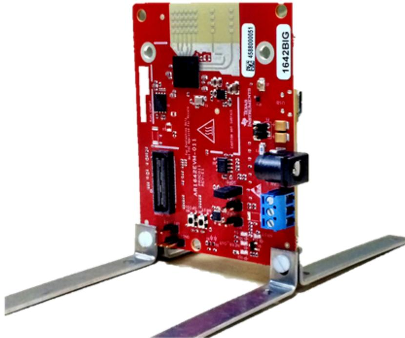
Figure 19. Vertical Assembly of EVM
