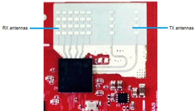
Figure 9. PCB Antennas
