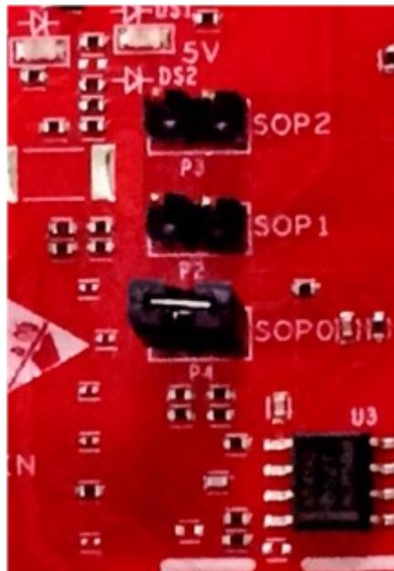
**Figure 11. SOP Jumpers**
