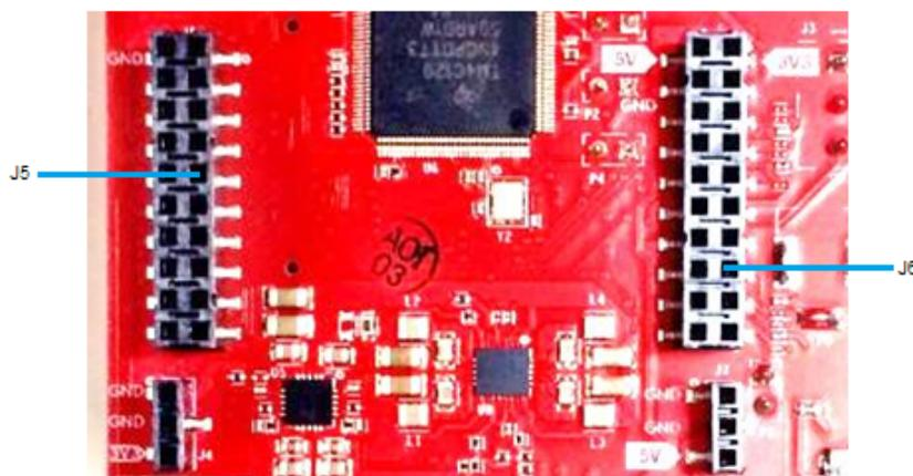
Figure 5. 20-Pin BoosterPack Connectors
