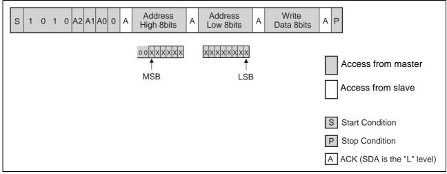
Note : In the MB85RC128A, input "00" as the upper 2 bits of the MSB.
