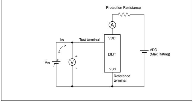
Note : The voltage V<sub>IN</sub> is increased gradually and the current I<sub>IN</sub> of 300 mA at maximum shall flow. Confirm the latch up does not occur under I<sub>IN</sub> =  $\pm$  300 mA. In case the specific requirement is specified for I/O and IIN cannot be 300 mA, the voltage shall be
