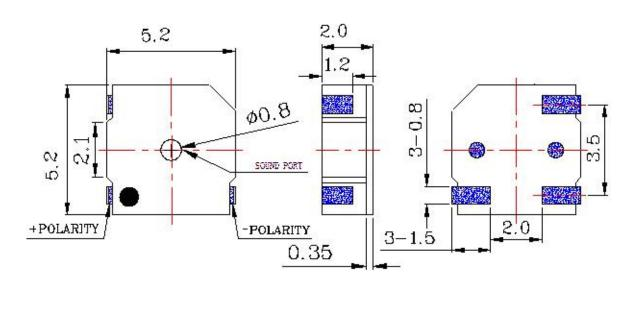
\*Unit: mm; Tolerance: ± 0.5mm Except Specified \*Housing Material: Black LCP \*Terminal plate: 3 soldering pads, tin Plating Brass
