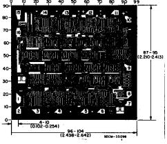
Dimensions and Pad Layout for CD4094B Chip.
