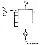
Fig. 17 — Quiescent device current test circuit.
