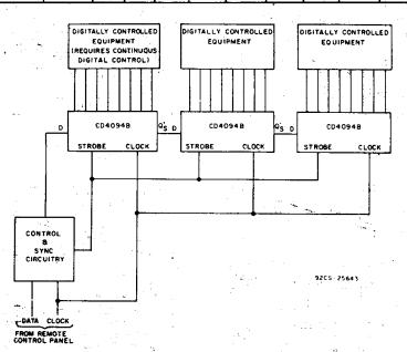
Fig. 14 - Remote control holding register.
