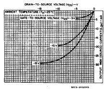
Fig. 6 - Typical output high (source) current characteristics.
