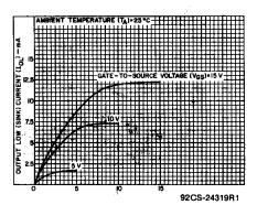
Fig. 5 - Minimum output low (sink) current characteristics.
