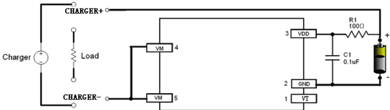
Fig 6 XB5352G in a Typical Battery Protection Circuit
