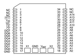
34-Pin PowerCap Module Board (Uses DS9034PCX PowerCap)
