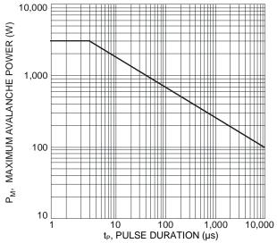
Fig. 8 Maximum Avalanche Power vs. Pulse Duration
