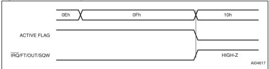
Figure 14. Backup mode alarm waveform
