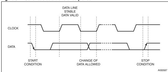
Figure 5. Serial bus data transfer sequence
