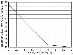
Figure 1. Typical Propagation Delay vs Supply Voltage
