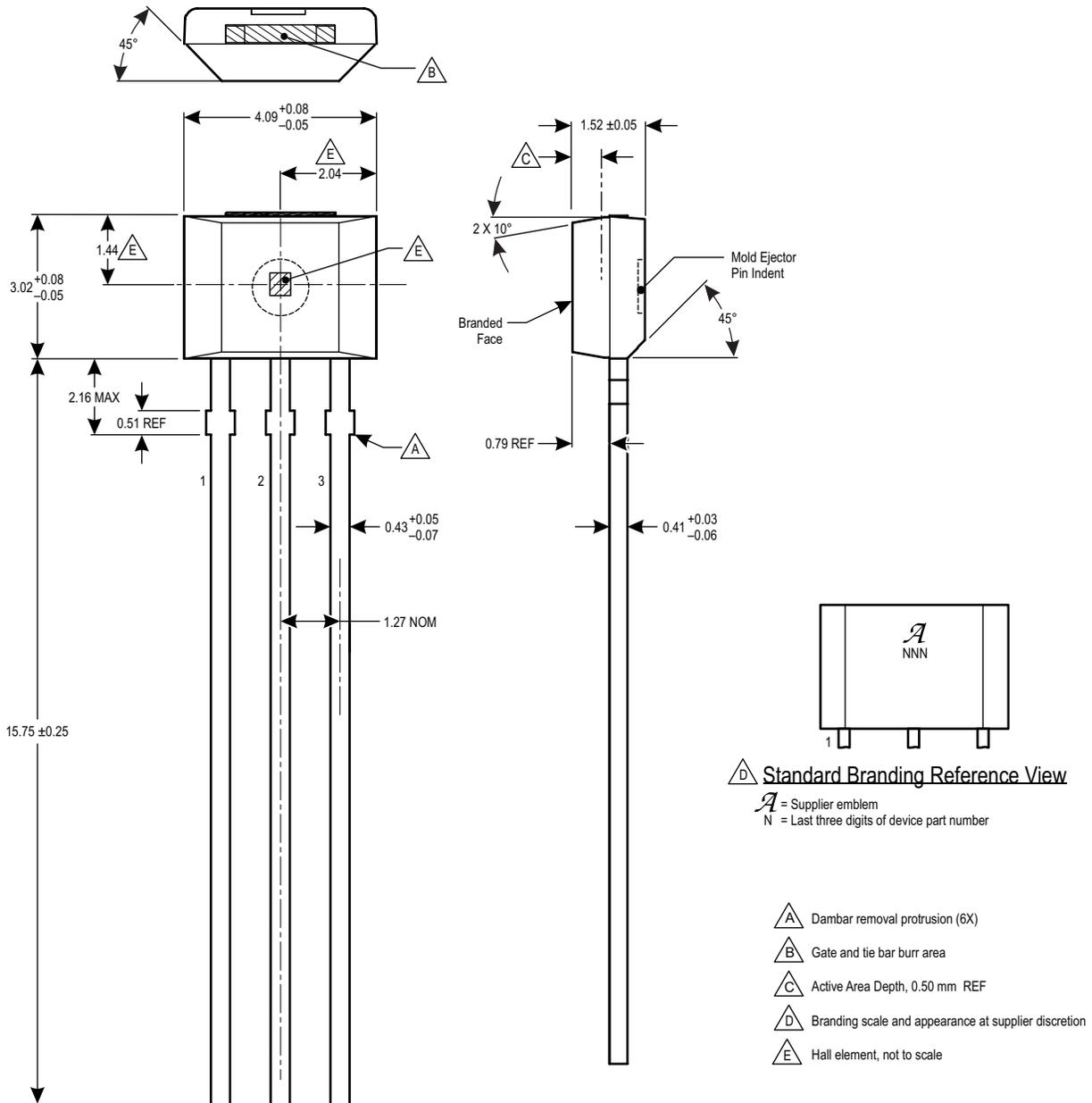
Figure 6: Package UA, 3-Pin SIP, Matrix Style
