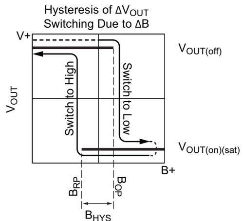
Figure 3: Output Voltage Responds to Magnetic Flux Density.
