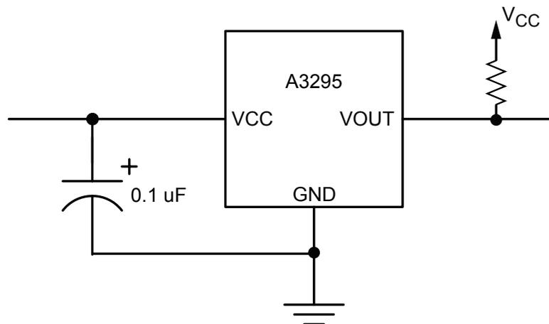
**Figure 4: Typical Basic Application Circuit**
