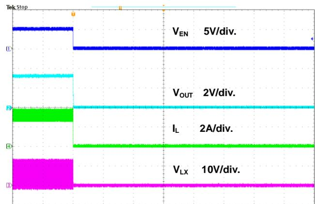
Figure 10. Power Off through  $\overline{SHDN}$  Waveform
