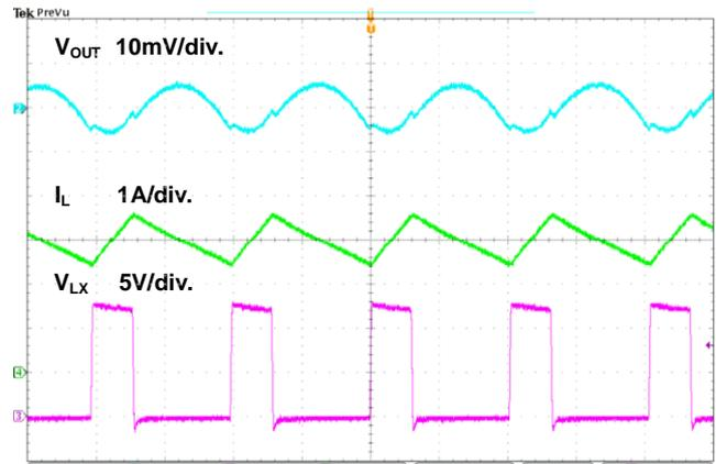
Figure 6. Steady State Waveform
