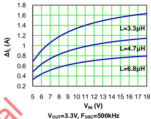
A good compromise value between size and efficiency is to set the peak-to-peak inductor ripple current  $\Delta I_L$  equal to 30% of the maximum load current. But setting the peak-to-peak inductor ripple current  $\Delta I_L$  between 20%~50% of the maximum load current is also acceptable. Then the inductance can be calculated with the following equation:
