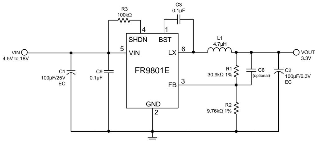
Figure 3. C<sub>IN</sub>/C<sub>OUT</sub> use Electrolytic Capacitors Application Circuit
