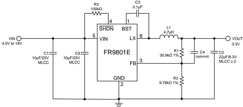
Figure 2. C<sub>IN</sub>/C<sub>OUT</sub> use Ceramic Capacitors Application Circuit
