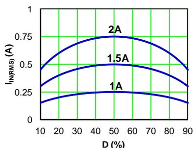
A low ESR capacitor is required to keep the noise minimum. Ceramic capacitors are better, but tantalum or low ESR electrolytic capacitors may also suffice. When using tantalum or electrolytic capacitors, a 0.1 $\mu$ F ceramic capacitor should be placed as close to the IC as possible.
