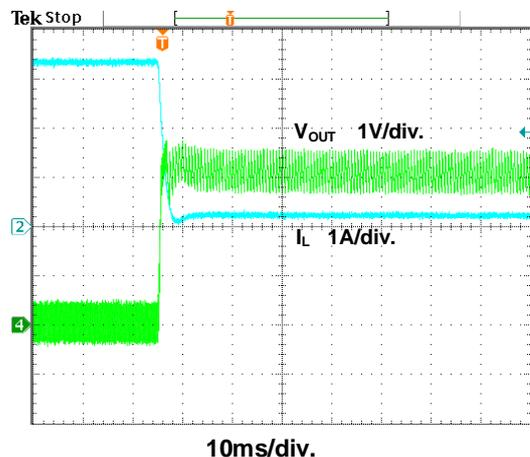
Figure 16. Short Circuit Test
