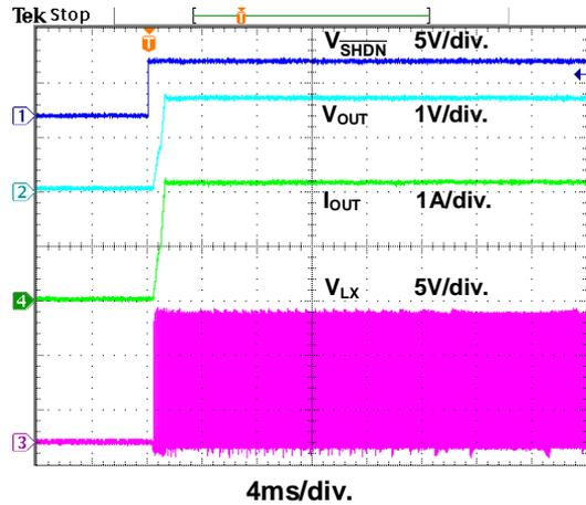
Figure 12. Power On through  $\overline{SHDN}$  Waveform
