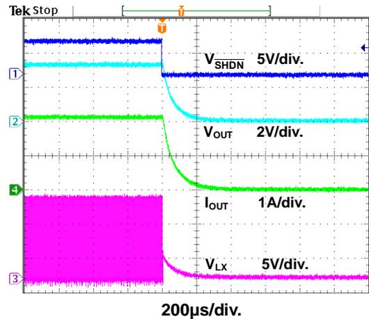
Figure 14. Power Off through  $\overline{SHDN}$  Waveform
