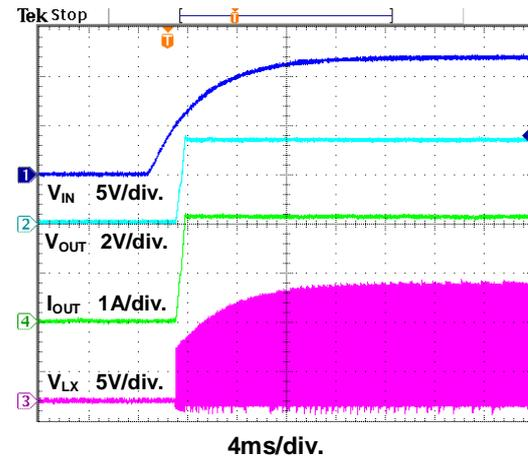
Figure 8. Power On through VIN Waveform
