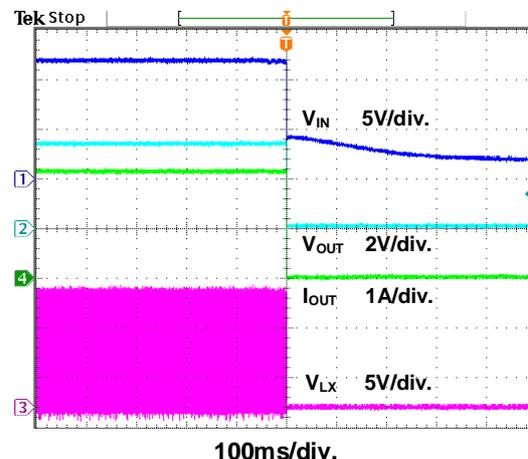
Figure 10. Power Off through VIN Waveform
