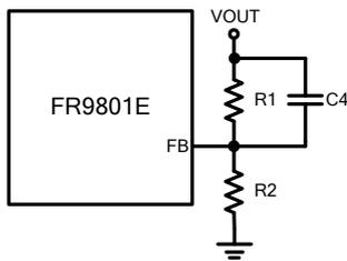
For optimizing the feedforward capacitor, knowing the cross frequency is the first thing. The cross frequency (or the converter bandwidth) can be determined by using a network analyzer. When getting the cross frequency with no feedforward capacitor identified, the value of feedforward capacitor C4 can be calculated with the following equation:
