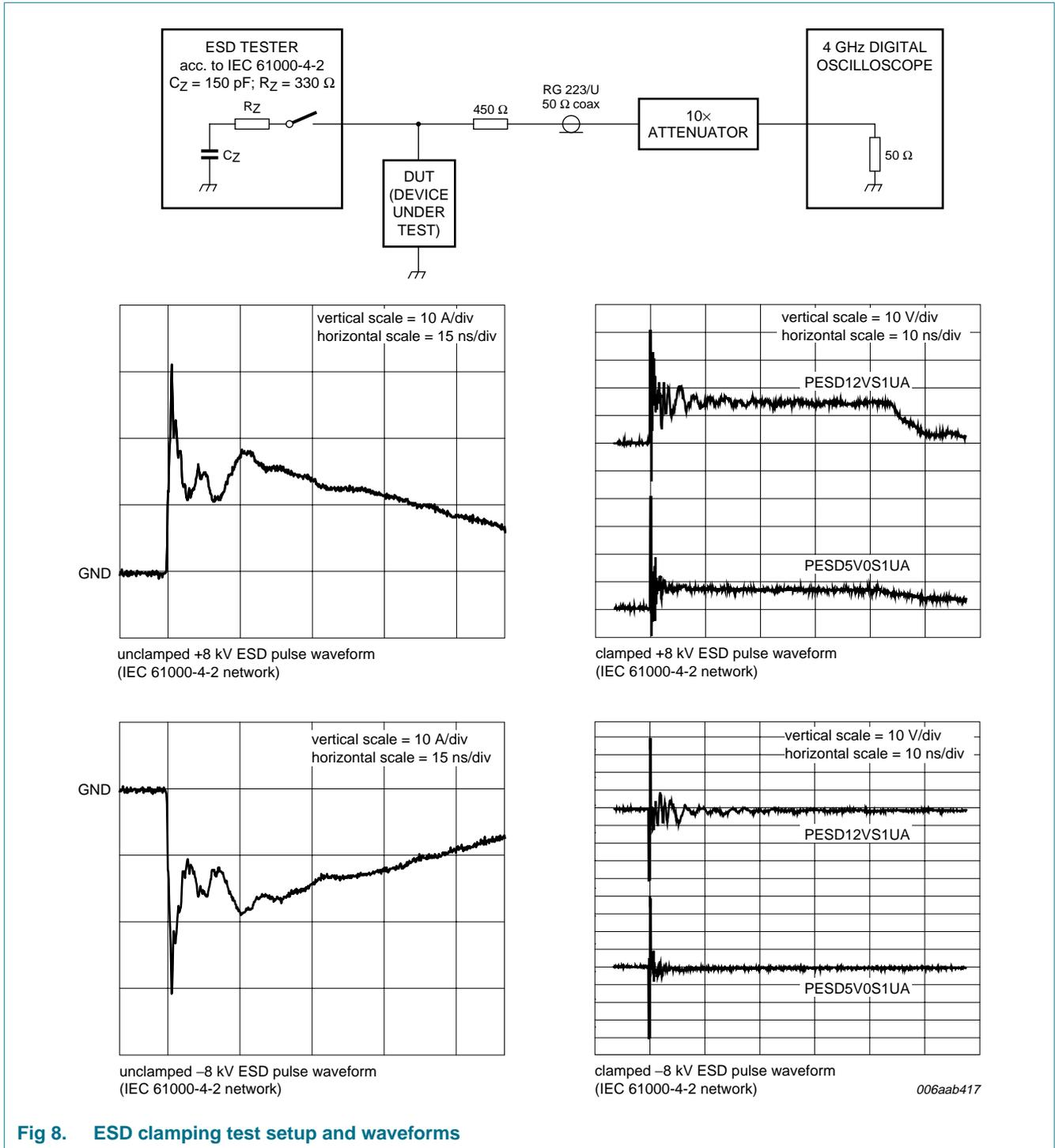
**Fig 8. ESD clamping test setup and waveforms**
