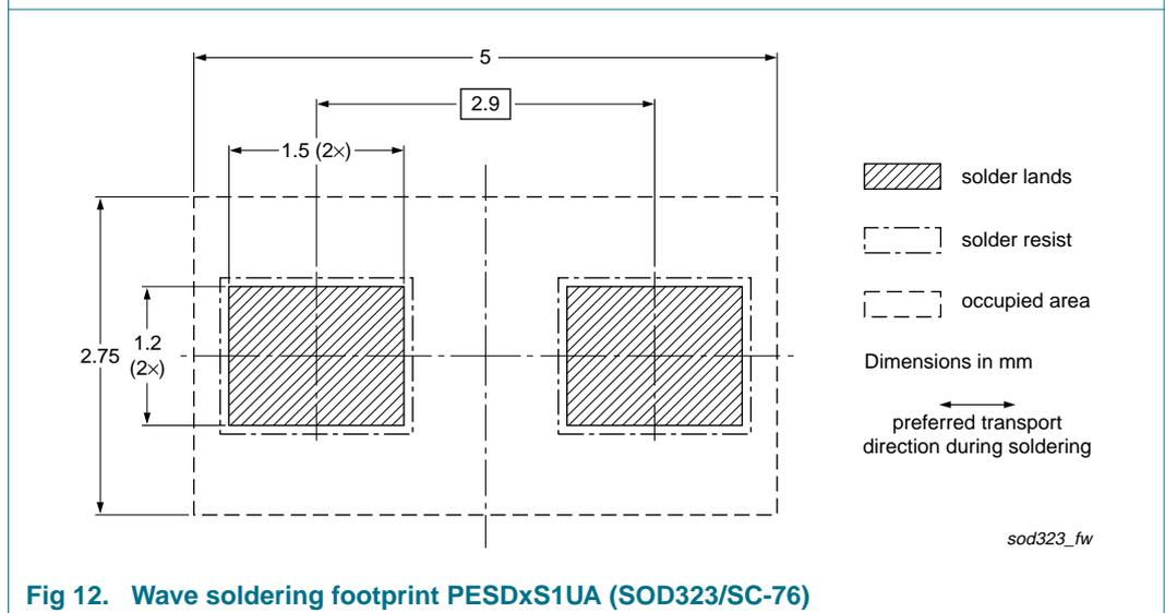
**Fig 12. Wave soldering footprint PESDxS1UA (SOD323/SC-76)**
