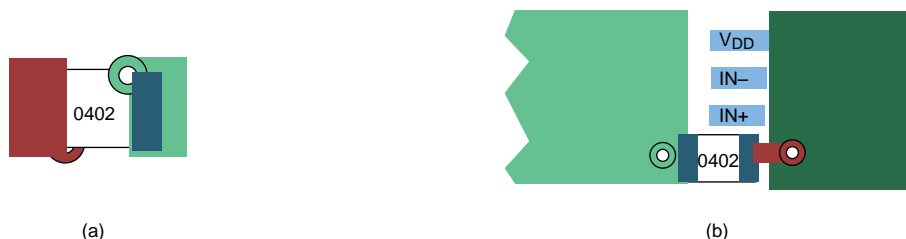
Figure 48. Typical Decoupling Capacitor Layouts
