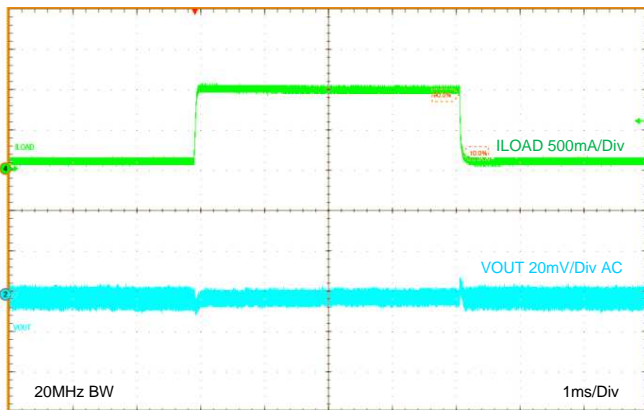
Figure 60. Load Transient V_{OUT} = 3.3\text{ V}
