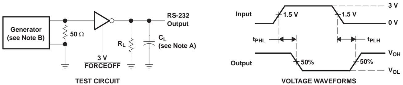
NOTES: A.  $C_L$  includes probe and jig capacitance.
