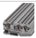
Feed-through terminal block, nom. voltage: 1000 V, nominal current: 41 A, connection method: Spring-cage connection, number of connections: 3, cross section:0.2 mm² - 10 mm², AWG: 24 - 8, width: 8.2 mm, color: gray, mounting type: NS 35/7,5, NS 35/15
