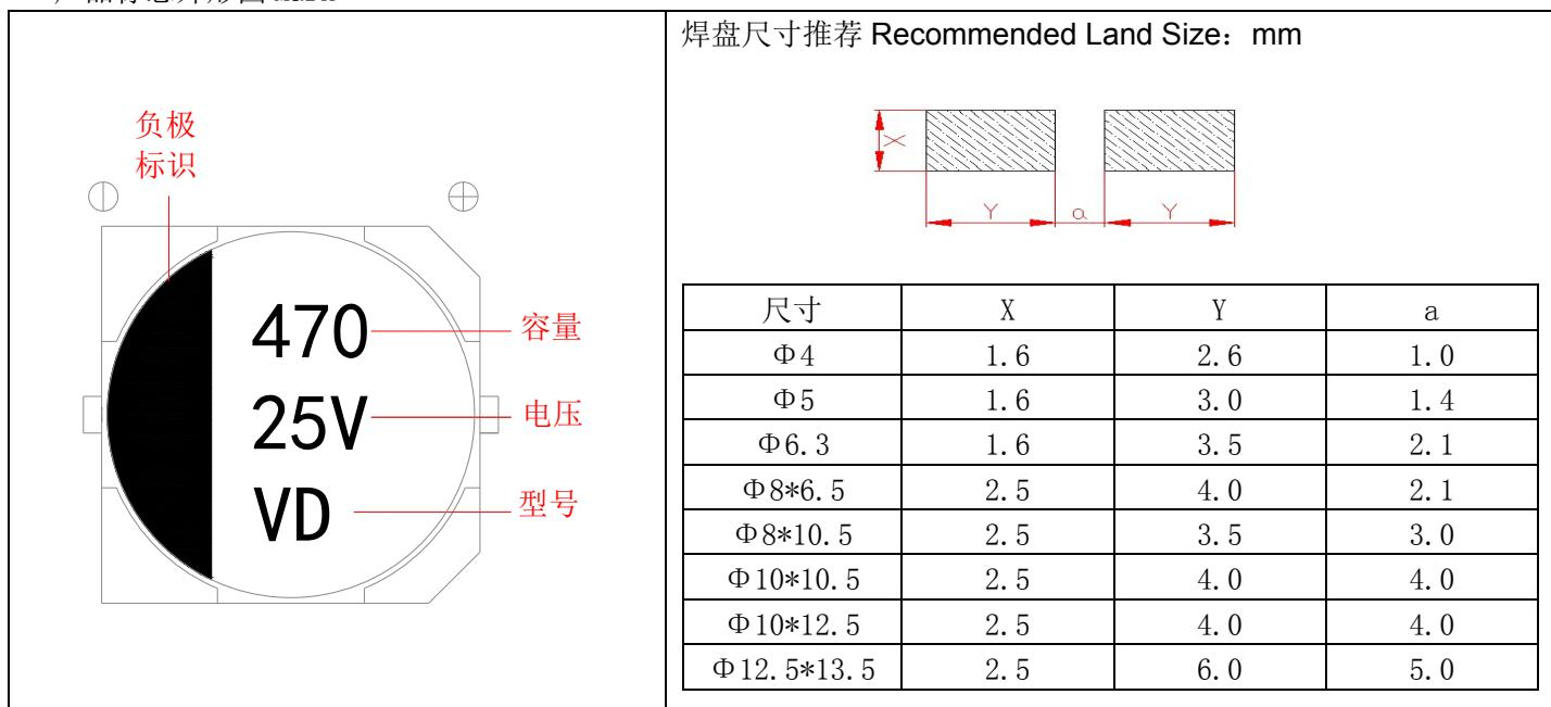
The diagram shows a circular capacitor with markings: a minus sign at the top left labeled '负极标识' (negative terminal indicator), a plus sign at the top right, '470' in the center labeled '容量' (capacity), '25V' below it labeled '电压' (voltage), and 'VD' at the bottom labeled '型号' (model). To the right is a table titled '焊盘尺寸推荐 Recommended Land Size: mm' showing dimensions X, Y, and a for various lead sizes.
