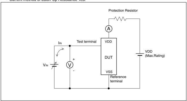
Note: The voltage  $V_{\text{IN}}$  is increased gradually and the current  $I_{\text{IN}}$  of 300 mA at maximum shall flow. Confirm the latch up does not occur under  $I_{\text{IN}} = \pm 300$  mA.
