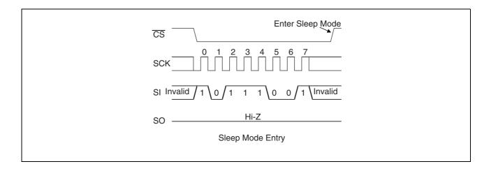
Returning to an normal operation from the SLEEP mode is carried out after  $t_{REC}$  (Max 400  $\mu s$ ) time from the falling edge of  $\overline{CS}$  (see the figure below). It is possible to return  $\overline{CS}$  to H level before  $t_{REC}$  time. However, it is prohibited to bring down  $\overline{CS}$  to L level again during  $t_{REC}$  period.
