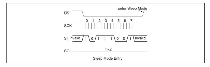
Returning to an normal operation from the SLEEP mode is carried out after tree (Max 400  $\mu$ s) time from the falling edge of  $\overline{CS}$  (see the figure below). It is possible to return  $\overline{CS}$  to H level before tree time. However, it is prohibited to bring down  $\overline{CS}$  to L level again during tree period.
