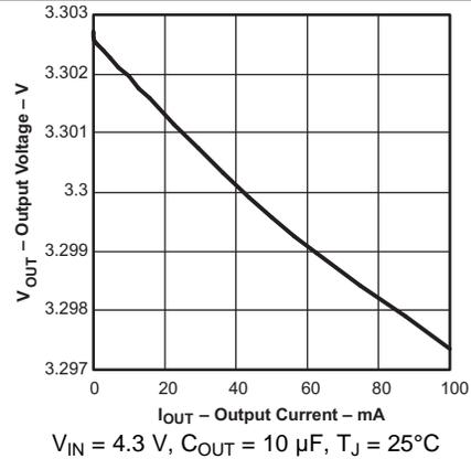
Figure 2. TPS79133 Output Voltage vs Output Current
