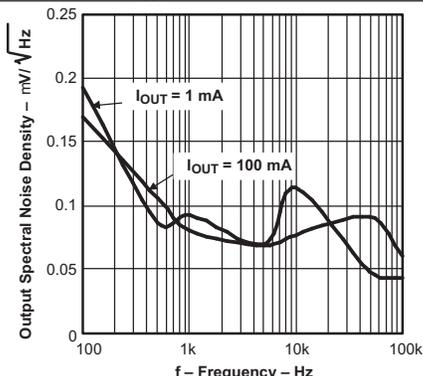
$V_{IN} = 2.8\text{ V}$ ,  $C_{OUT} = 10\text{ }\mu\text{F}$ ,  $C_{BYPASS} = 0.1\text{ }\mu\text{F}$
