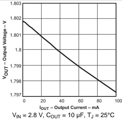
Figure 1. TPS79118 Output Voltage vs Output Current
