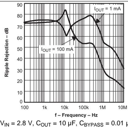
Figure 18. TPS79118 Ripple Rejection vs Frequency
