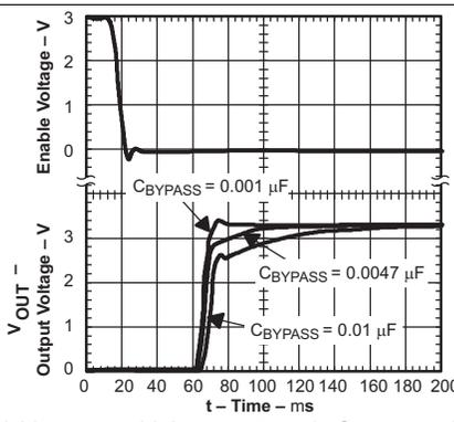
$V_{IN} = 4.3\text{ V}$ ,  $V_{OUT} = 3.3\text{ V}$ ,  $I_{OUT} = 100\text{ mA}$ ,  $C_{OUT} = 1\text{ }\mu\text{F}$ ,  $T_J = 25^\circ\text{C}$
