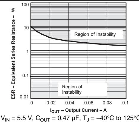
Figure 29. TPS79118 Typical Regions of Stability Equivalent Series Resistance (ESR) vs Output Current
