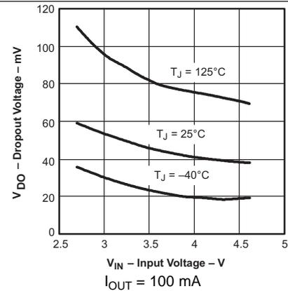
Figure 16. TPS79101 Dropout Voltage vs Input Voltage
