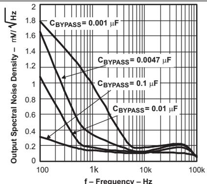
$V_{IN} = 4.3\text{ V}$ ,  $I_{OUT} = 100\text{ mA}$ ,  $C_{OUT} = 10\text{ }\mu\text{F}$
