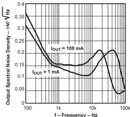
$V_{IN} = 4.3\text{ V}$ ,  $C_{OUT} = 10\text{ }\mu\text{F}$ ,  $C_{BYPASS} = 0.1\text{ }\mu\text{F}$
