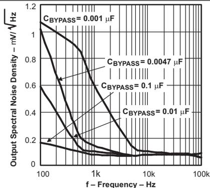
$V_{IN} = 2.8\text{ V}$ ,  $I_{OUT} = 100\text{ mA}$ ,  $C_{OUT} = 10\text{ }\mu\text{F}$
