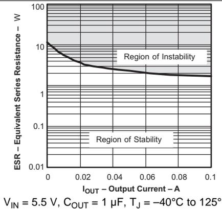
Figure 30. TPS79118 Typical Regions of Stability Equivalent Series Resistance (ESR) vs Output Current
