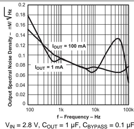
Figure 6. TPS79118 Output Spectral Noise Density vs Frequency
