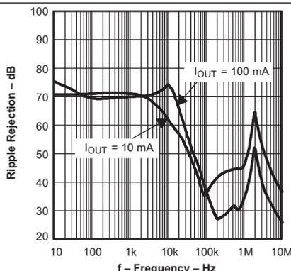
$V_{IN} = 4.3\text{ V}$ ,  $C_{OUT} = 1\text{ }\mu\text{F}$ ,  $C_{BYPASS} = 0.01\text{ }\mu\text{F}$
