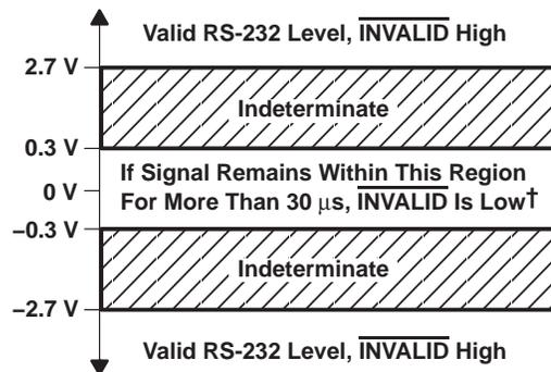
† Auto-powerdown disables drivers and reduces supply current to 1  $\mu\text{A}$ .
