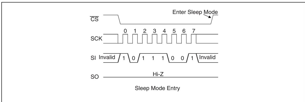
Returning to a normal operation from the SLEEP mode is carried out after  $t_{REC}$  (Max 400  $\mu$ s) time from the falling edge of  $\overline{CS}$  (see the figure below). It is possible to return  $\overline{CS}$  to H level before  $t_{REC}$  time. However, it is prohibited to bring down  $\overline{CS}$  to L level again during  $t_{REC}$  period.
