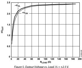
Figure 5. Output Voltage vs. Load,  $V_s = \pm 2.5 V$  $R_{LOAD}$  is Connected to GND (0 V)
