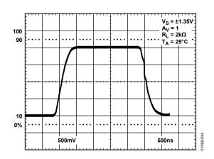
Figure 34. Large Signal Transient Response
