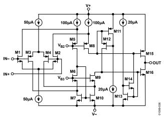
Figure 36. Simplified Equivalent Circuit
