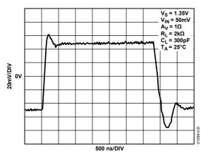
Figure 31. Small Signal Transient Response
