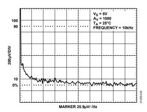
Figure 20. Voltage Noise Density vs. Frequency (10 kHz)
