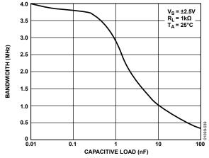
Figure 39. Unity-Gain Bandwidth vs. Capacitive Load
