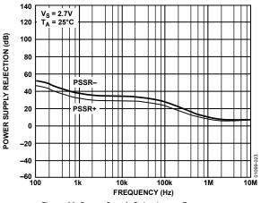
Figure 23. Power Supply Rejection vs. Frequency
