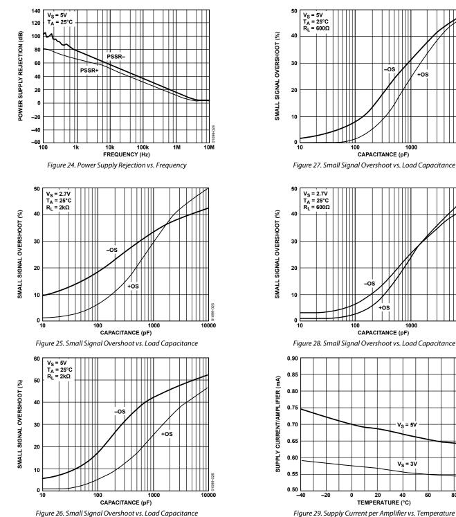
Figure 29. Supply Current per Amplifier vs. Temperature
