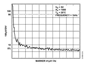
Figure 19. Voltage Noise Density vs. Frequency (1 kHz)
