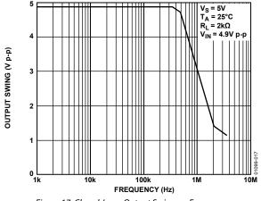
Figure 17. Closed-Loop Output Swing vs. Frequency
