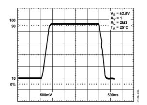
Figure 33. Large Signal Transient Response
