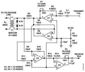
Figure 46. Single-Supply Direct Access Arrangement for Modems
