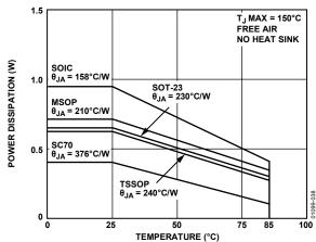
Figure 38. Maximum Power Dissipation vs. Ambient Temperature
