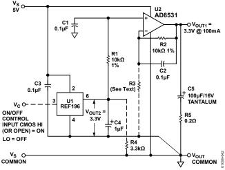
Figure 42. High Output Current Reference/Regulator
