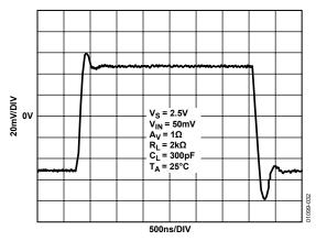
Figure 32. Small Signal Transient Response
