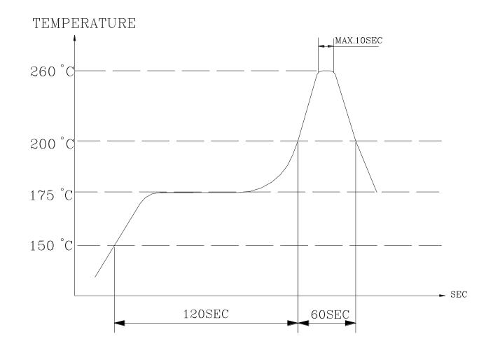
Heat resistant line (Used when heat resistant reliablity test is performed) (2)Manual soldering Manual soldering temperature 350 °C within 10 sec.
