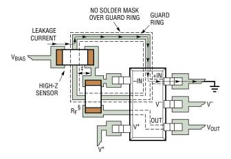
$\ddagger$  NO LEAKAGE CURRENT, V\_IN = V\_1IN  $\S$  AVOID DISSIPATING SIGNIFICANT AMOUNTS OF POWER IN THIS RESISTOR. IT WILL GENERATE THERMAL GRADIENTS WITH RESPECT TO THE INPUT PINS AND LEAD TO THERMOCOUPLE-INDUCED ERROR. THERMALLY ISOLATE OR ALIGN WITH INPUTS IF RESISTOR WILL CAUSE HEATING.
