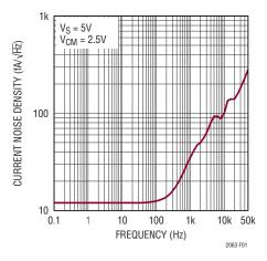
Figure 1. Input Current Noise Spectrum
