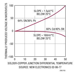
Figure 3. Solder-Copper Thermal EMFs
