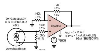
Figure 9. Micropower Precision Oxygen Sensor
