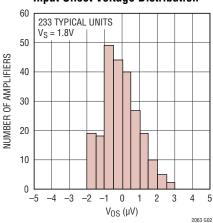
**Input Offset Voltage Drift** Distribution
