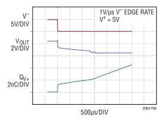
Figure 6. Charge Loss During Power-Up
