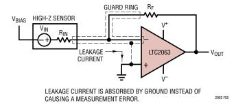
Figure 5. Example Layout of Inverting Amplifier with Leakage Guard Ring
