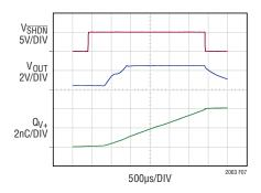
Figure 7. Charge Loss Due to Enabling and Disabling via SHDN Pin
