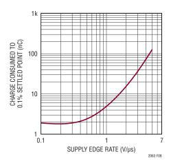
Figure 8. Power-Up Charge vs Supply Edge Rate
