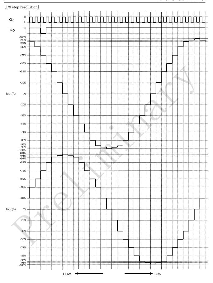
$\operatorname{MO}$  output shown in the timing chart is when the  $\operatorname{MO}$  pin is pulled up.
