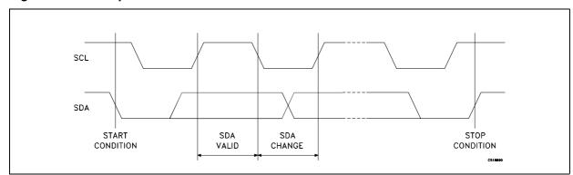
Figure 12. Basic operation of the I<sup>2</sup>C Bus
