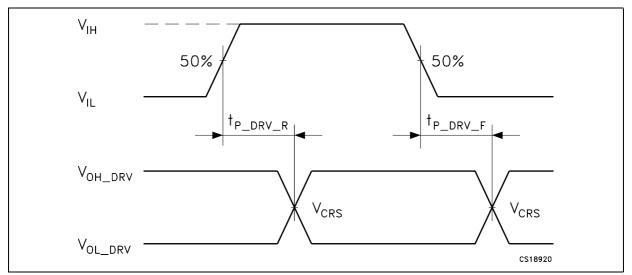
Figure 7. Differential receiver propagation delay
