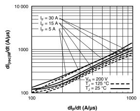
Fig. 8 - Typical dl<sub>(rec)M</sub>/dt vs. dl<sub>F</sub>/dt
