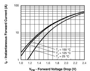
Fig. 1 - Maximum Forward Voltage Drop vs. Instantaneous Forward Current
