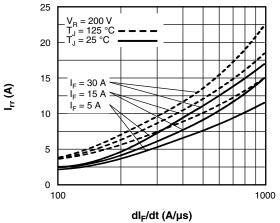
Fig. 6 - Typical Recovery Current vs. dl<sub>F</sub>/dt
