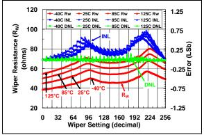
**FIGURE 2-9:** 5 kΩ Rheo Mode –  $R_W$  (Ω), INL (LSb), DNL (LSb) vs. Wiper Setting and Ambient Temperature ( $V_{DD}$  = 5.5V).
