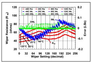
**FIGURE 2-37:** 100  $k\Omega$  Pot Mode –  $R_W$  ( $\Omega$ ), INL (LSb), DNL (LSb) vs. Wiper Setting and Ambient Temperature ( $V_{DD}$  = 5.5V).
