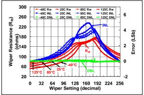
**FIGURE 2-10:** 5 kΩ Rheo Mode –  $R_W$  (Ω), INL (LSb), DNL (LSb) vs. Wiper Setting and Ambient Temperature ( $V_{DD}$  = 3.0V).
