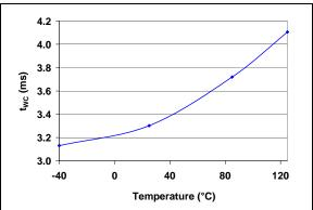
**FIGURE 2-55:** Nominal EEPROM Write Cycle Time vs. V<sub>DD</sub> and Temperature.
