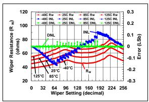
**FIGURE 2-27:** 50 k $\Omega$  Pot Mode –  $R_W$  ( $\Omega$ ), INL (LSb), DNL (LSb) vs. Wiper Setting and Ambient Temperature ( $V_{DD} = 5.5V$ ).
