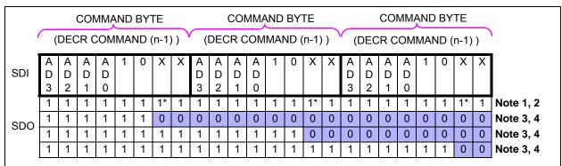
Note 1: Only functions when writing the volatile wiper registers (AD3:AD0) 0h and 1h.
