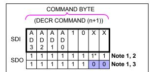
**Note 1:** Only functions when writing the volatile wiper registers (AD3:AD0) 0h and 1h.
