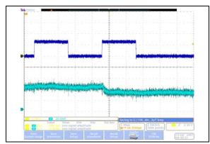
**FIGURE 2-23:** 10 kΩ – Low-Voltage Decrement Wiper Settling Time ( $V_{DD} = 2.7V$ ) (1 μs/Div).
