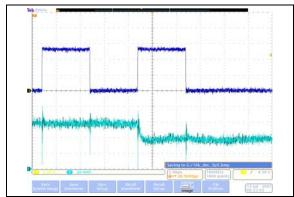
**FIGURE 2-24:** 10 kΩ – Low-Voltage Decrement Wiper Settling Time ( $V_{DD} = 5.5V$ ) (1 μs/Div).
