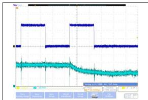
**FIGURE 2-44:** 100 kΩ – Low-Voltage Decrement Wiper Settling Time ( $V_{DD} = 5.5V$ ) (1 μs/Div).
