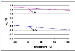
**FIGURE 2-52:**  $V_{IL}$  (SDI, SCK,  $\overline{CS}$ ,  $\overline{WP}$ , and SHDN) vs.  $V_{DD}$  and Temperature.
