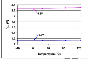
**FIGURE 2-51:**  $V_{IH}$  (SDI, SCK,  $\overline{CS}$ ,  $\overline{WP}$ , and SHDN) vs.  $V_{DD}$  and Temperature.
