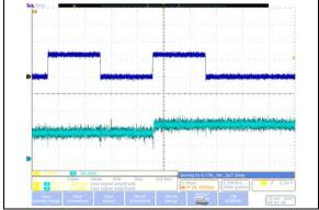
**FIGURE 2-15:**  $5 k\Omega - Low$ -Voltage Increment Wiper Settling Time ( $V_{DD} = 2.7V$ ) (1  $\mu$ s/Div).
