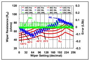
**FIGURE 2-6:**  $5 \text{ } k\Omega \text{ Pot Mode} - R_W (\Omega),$  INL (LSb), DNL (LSb) vs. Wiper Setting and Ambient Temperature ( $V_{DD} = 5.5V$ ).
