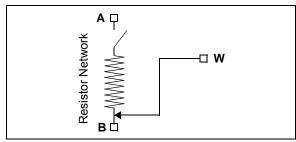
**FIGURE 5-2:** Hardware Shutdown Resistor Network Configuration.
