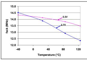
**FIGURE 2-57:** SCK Input Frequency vs. Voltage and Temperature.
