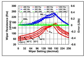
**FIGURE 2-41:** 100 kΩ Rheo Mode –  $R_W$  (Ω), INL (LSb), DNL (LSb) vs. Wiper Setting and Ambient Temperature ( $V_{DD}$  = 3.0V).
