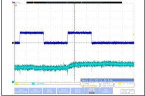
**FIGURE 2-35:** 50 k $\Omega$  – Low-Voltage Increment Wiper Settling Time ( $V_{DD}$  = 2.7V) (1  $\mu$ s/Div).
