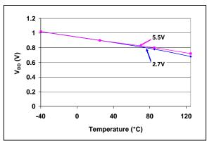
**FIGURE 2-56:** POR/BOR Trip point vs.  $V_{DD}$  and Temperature.
