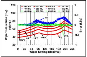
**FIGURE 2-20:** 10  $k\Omega$  Rheo Mode –  $R_W(\Omega)$ , INL (LSb), DNL (LSb) vs. Wiper Setting and Ambient Temperature ( $V_{DD} = 5.5V$ ).
