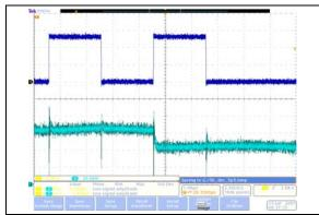
**FIGURE 2-13:** 5 kΩ – Low-Voltage Decrement Wiper Settling Time ( $V_{DD} = 5.5V$ ) (1 μs/Div).
