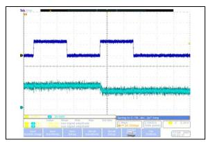
**FIGURE 2-12:**  $5 \text{ k}\Omega - \text{Low-Voltage}$  Decrement Wiper Settling Time ( $V_{DD} = 2.7V$ ) (1  $\mu$ s/Div).
