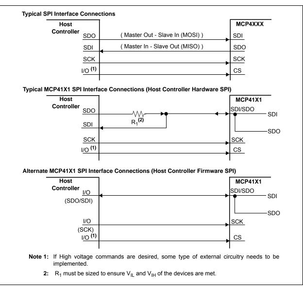
FIGURE 6-1: Typical SPI Interface Block Diagram.
