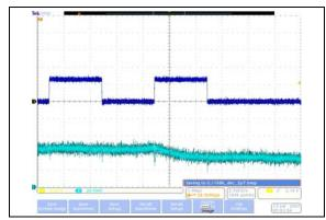
**FIGURE 2-43:** 100 k $\Omega$  – Low-Voltage Decrement Wiper Settling Time ( $V_{DD}$  = 2.7V) (1  $\mu$ s/Div).
