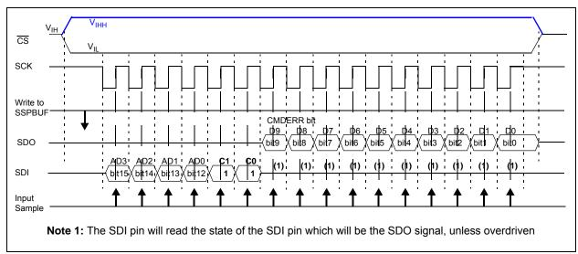
**FIGURE 6-5:** 16-Bit Read Command for Devices with SDI/SDO multiplexed - SPI Waveform (Mode 1,1).
