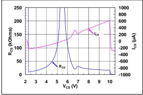
**FIGURE 2-4:**  $\overline{\text{CS}}$  Pull-up/Pull-down Resistance ( $R_{\overline{\text{CS}}}$ ) and Current ( $I_{\overline{\text{CS}}}$ ) vs.  $\overline{\text{CS}}$  Input Voltage ( $V_{\overline{\text{CS}}}$ ) ( $V_{DD} = 5.5V$ ).
