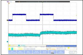
**FIGURE 2-25:** 10  $k\Omega$  – Low-Voltage Increment Wiper Settling Time ( $V_{DD}$  = 2.7V) (1  $\mu$ s/Div).
