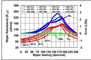
**FIGURE 2-21:** 10  $k\Omega$  Rheo Mode –  $R_W(\Omega)$ , INL (LSb), DNL (LSb) vs. Wiper Setting and Ambient Temperature ( $V_{DD} = 3.0V$ ).
