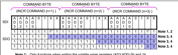
Note 1: Only functions when writing the volatile wiper registers (AD3:AD0) 0h and 1h.
