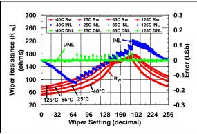
**FIGURE 2-28:** 50 kΩ Pot Mode –  $R_W$  (Ω), INL (LSb), DNL (LSb) vs. Wiper Setting and Ambient Temperature ( $V_{DD}$  = 3.0V).
