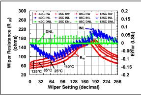
**FIGURE 2-38:** 100 k $\Omega$  Pot Mode –  $R_W$  ( $\Omega$ ), INL (LSb), DNL (LSb) vs. Wiper Setting and Ambient Temperature ( $V_{DD} = 3.0V$ ).
