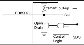
FIGURE 6-2: Serial I/O Mux Block Diagram.
