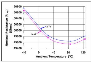
**FIGURE 2-29:** 50 k $\Omega$  – Nominal Resistance ( $\Omega$ ) vs. Ambient Temperature and V<sub>DD</sub>.
