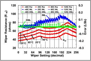
**FIGURE 2-40:** 100 kΩ Rheo Mode –  $R_W$  (Ω), INL (LSb), DNL (LSb) vs. Wiper Setting and Ambient Temperature ( $V_{DD}$  = 5.5V).
