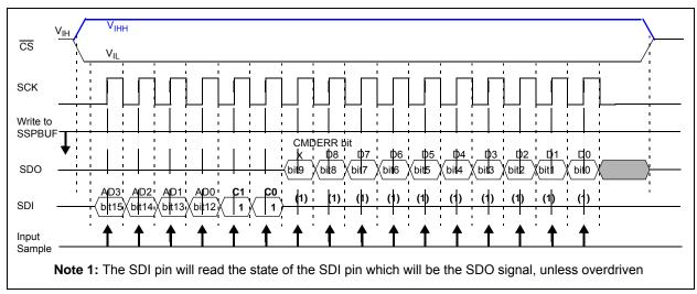
**FIGURE 6-6:** 16-Bit Read Command for Devices with SDI/SDO multiplexed - SPI Waveform (Mode 0,0).
