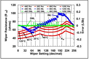
**FIGURE 2-30:** 50  $k\Omega$  Rheo Mode –  $R_W(\Omega)$ , INL (LSb), DNL (LSb) vs. Wiper Setting and Ambient Temperature ( $V_{DD} = 5.5V$ ).
