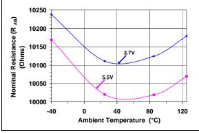
**FIGURE 2-19:** 10 k $\Omega$  – Nominal Resistance ( $\Omega$ ) vs. Ambient Temperature and V<sub>DD</sub>.
