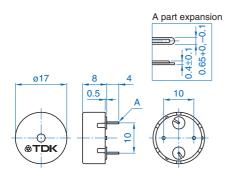
Tolerance: ±0.3 Dimensions in mm
