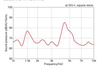
\* The frequency characteristic changes depending on the case shape and the installation method.
